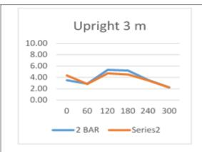
Fig. 7. U pright sprinkler Discharge Density variation when installed at 3 m with 2 bar and 2.5 bar pressure
