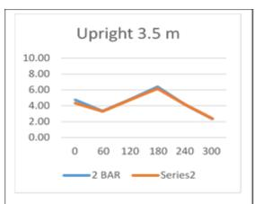
Fig. 8. U pright sprinkler Discharge Density variation when installed at 3.5 m with 2 bar and 2.5 bar pressure
