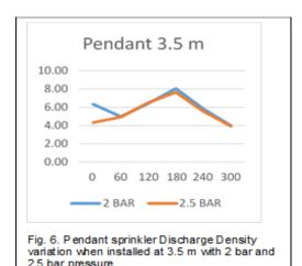
From the Fig No.6, It is found that, discharge density is initially decreasing from the centre value till 60 cm radial diatnace and then increasing till 180 cm radial distance and then de-
