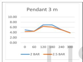
Fig. 5. Pendant sprinkler Discharge Density variation when installed at 3 m with 2 bar and 2.5 bar pressure
